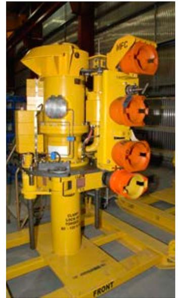
MARS system permanent injection choke
