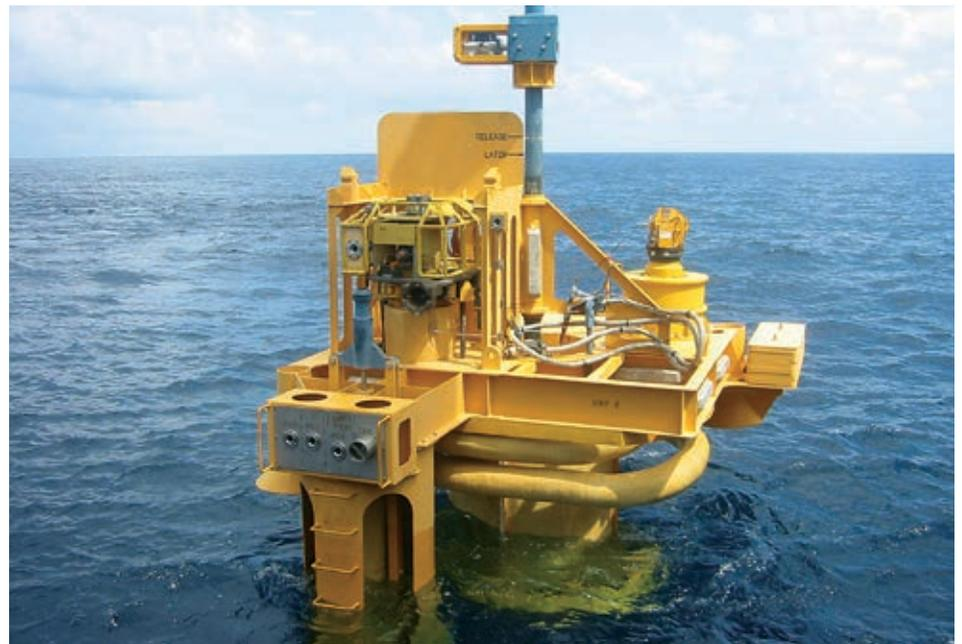
The MARS system enables the retrofit of a variety of production-enhancing technologies. This particular module was deployed onto existing wet subsea trees, enabling subsea multiphase pumping.
