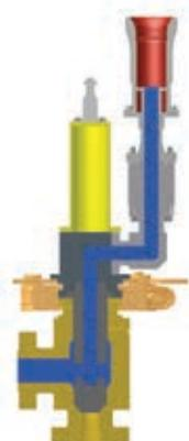
MARS system injection insert (wellbore flow path)
