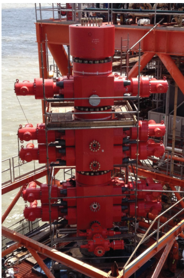
This 25,000-psi BOP stack was run in the Gulf of Mexico in 2012. A single 70,000-lb BOP body required eight months to forge and machine. (Source: Cameron)
