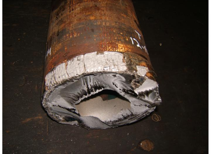
*The BroadShear rams are the industry's only technology that can successfully shear tool joint hard banding (above) and drillpipe forced to the side of the BOP (below).*
