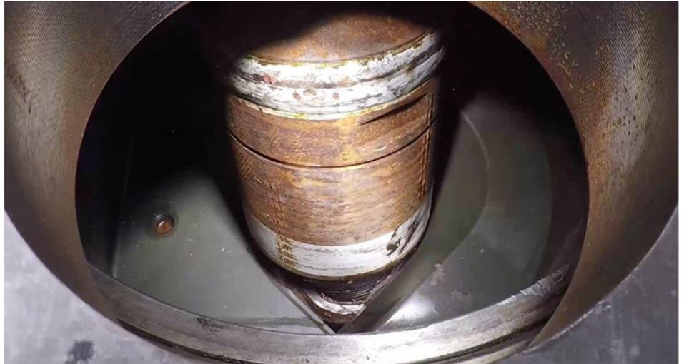
*In a series of rigorous tests, BroadShear rams demonstrated their ability to shear casing diameters up to 16 in, tool joint hardbanding, and off-center tubulars, which have long been considered unshearable using conventional technology.*
